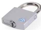
Cylinder padlock no. 215 N/58 WSM Stainless steel shackle Housing 58 mm wide, 50 mm high Latches without locking Shackle clearance 35 mm (standard)
