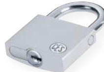
Cylinder padlock No. 215 N Stainless steel shackle Housing 58 mm wide, 50 mm high Latches without locking Shackle clearance 35 mm
