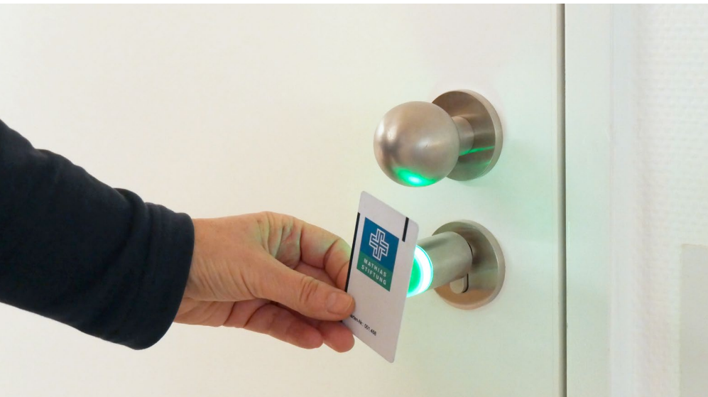
Access authorisation to an electronic cylinder with wireless installation. No alterations to the doors were required when changing from the mechanical locking system to the access control system. A mechanical cylinder was simply replaced by an electronic cylinder.
