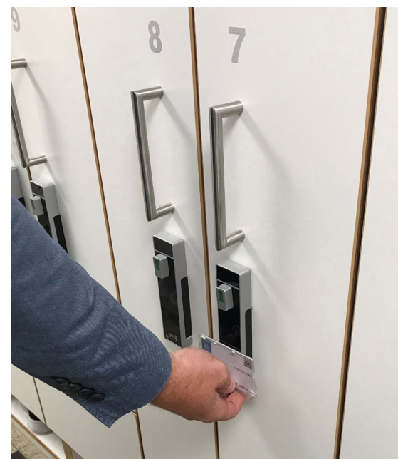
AccessOne software offers a wide range of settings for the use of RFID furniture locks. In the staff changing areas, the locks are programmed so that an employee can occupy a vacant locker for 12 hours.
