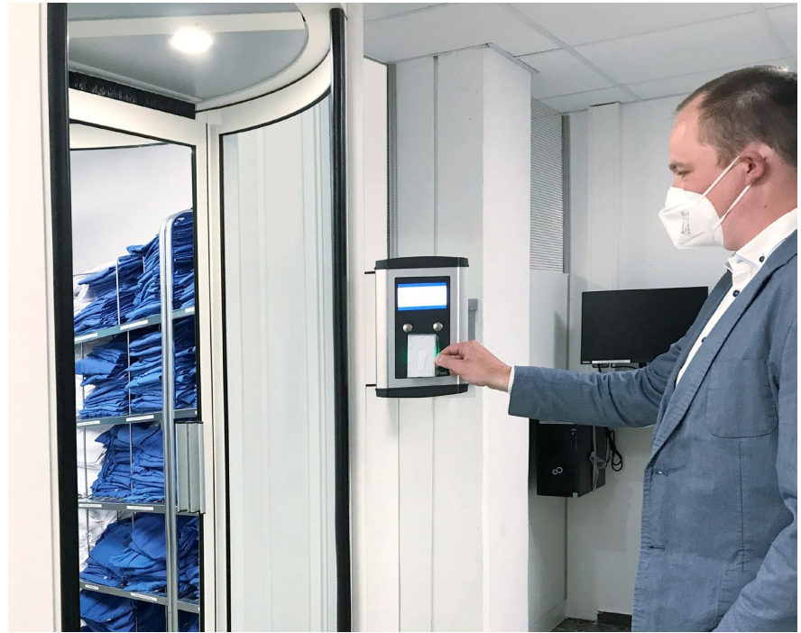
Authentication for the KEMAS laundry system is provided via the employee's ID card. Collection and return of the laundry are logged in the KEMAS system.
