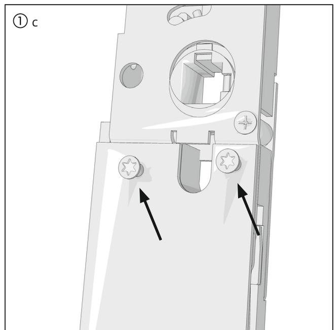
Select the matching dead bolt head for the backset. Push the dead bolt head onto the dead bolt plate and fasten it with a **M3x6** flat head screw.
