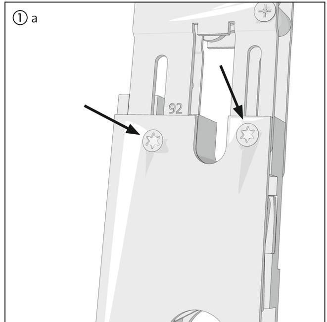
Next tighten the screws on the front face again. To facilitate the subsequent fitting of the forend (step 7), only tighten the screws slightly at this stage.
