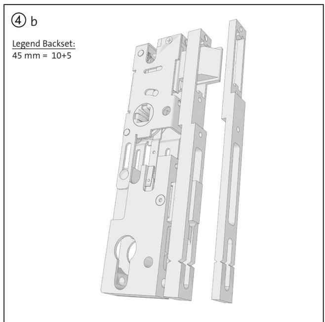
Select the desired forend. We recommend using the old forend as a template for drilling the fastening holes. Use the fixing screw hole for the alignment.
