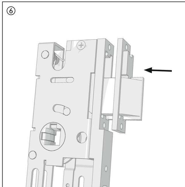
Place the desired forend, slightly tighten the screws and check the dead bolt function.
