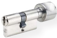
Knob cylinder no. 815 PXM Brass, satin nickel-plated Locking function on one side, aluminum knob on the other side, NF, various knob shapes available (figure shows shape H)
