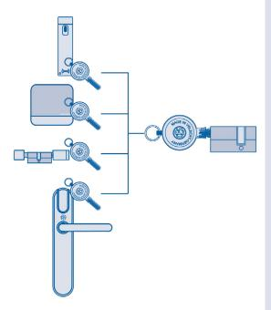
master key systems with electronic devices and identical locking medium technology. This enables the electronic key to also be used in other systems, such as lift control systems, for time registration or for payment systems.
