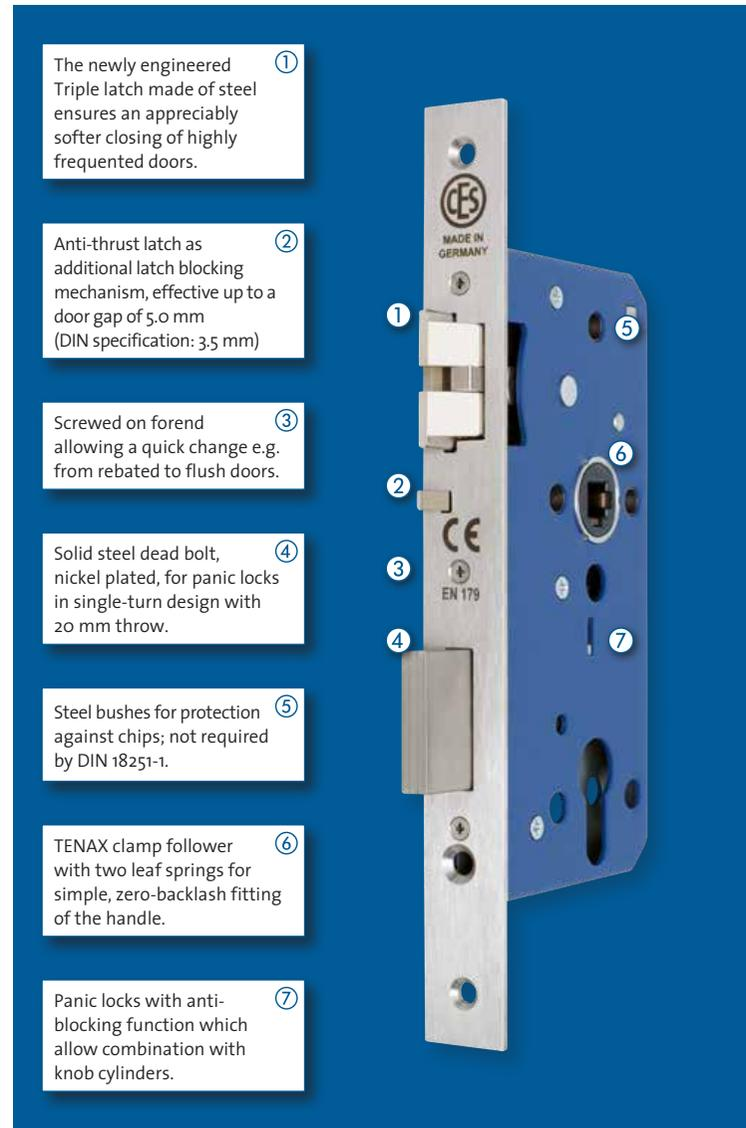
① The newly engineered Triple latch made of steel ensures an appreciably softer closing of highly frequented doors.
