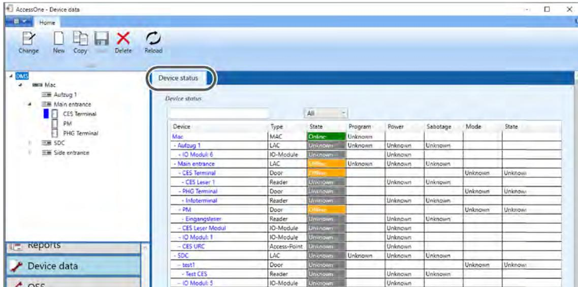
AccessOne provides a device data editor for the creation and parametrisation of devices. This shows the devices in a tree structure in the object selection on the left. The top entry is the Data Management System (DMS), and the devices are arranged beneath this. All of the data changes and all of the messages from door controllers (TSG1, TSG8, AMC or LAC\*) are completed here. This is therefore also where the status messages are interpreted, stored in the memory and displayed.
