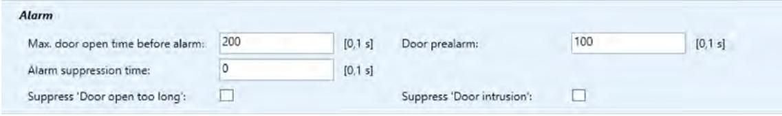
**Max. door open time before alarm:** Defines how long the system should wait for the door to be closed again before an alarm is issued. This value is specified in tenths of a second. If the specified time is exceeded, the system generates a log entry with the text 'Door open too long'.
