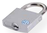
Cylinder padlock no. 215 N/58 UDM Stainless steel shackle Housing 58 mm wide, 50 mm high Latches without locking Shackle clearance 35 mm (standard)
