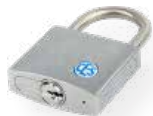
Cylinder padlock no. 215 N/58 PSM Lock case brass chromium velour finish Shackle stainless steel Case width 58 mm, height 50 mm Key removable without locking Shackle clearance 35 mm (standard)
