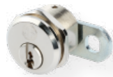
Cam cylinder no. 5558/30 PSM Brass, polished nickel plated Locking movement 90° Locking direction as desired Fitting dimension 25 mm
