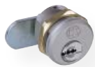
Cam cylinder no. 5558/30 WSM Brass, polished nickel plated Locking movement 90° Locking direction as desired Fitting dimension 25 mm
