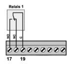
Connect the swing door drive with the screw terminals 17 and 19 on terminal strip 4.
