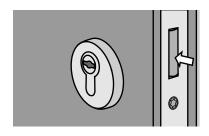
The dead bolt is retracted and the latch bolt is pulled in for a short period.
