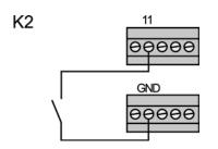
If this contact is closed, the door is permanently unlocked and the latch is pulled back. This status is independent of the selected mode of operation (Daytime mode or Nighttime mode).
