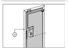
▶ Do not connect the shielding with the motor unit housing.
