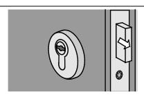
The dead bolt moves into the position defined by the wiring (Daytime/Nighttime mode). This ends the Learning mode.
