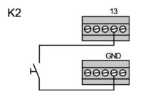
This function serves to unlock the door. If this contact is closed, the door is unlocked. This status is independent of the selected mode of operation (Daytime mode or Nighttime mode), with the exception of Permanent Open mode.
