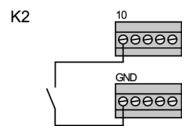
If this contact is closed, the door is locked, irrespective of the selected mode of operation (Daytime mode or Nighttime mode).
