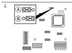
Plug the jumper into "configuration" position (pos. A in the figure).
