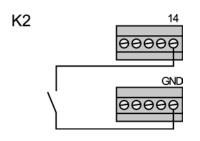
This input must always be connected to a door contact as malfunctions of the motor cylinder may occur otherwise.
