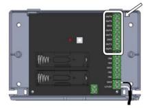
The communication module is equipped with 6 outputs labelled OUT1 to OUT6.
