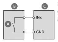
Between INx and GND a potential-free contact is connected (e.g. a switch or a relay). As soon as the contact closes, INx is considered to be 'active'.
