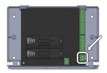
**3. Connect the power supply unit (see** "How to connect the power supply unit" **on page 14).**
