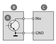
A device with an open-collector output is connected to INx of the communication module. As soon as the output is activated, INx is considered to be 'active'.
