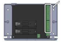
**4. Connect the inputs and outputs (see** "How to connect the inputs and outputs" **on page 15).**
