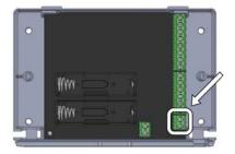
The port intended for connection of the power supply unit is located at the screw terminal marked "12VCD" and "GND".
