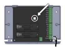
2. Press the coupling button of the communication module for approx. 1 second.
