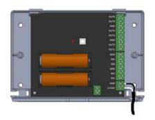
2. If necessary, take out the two empty batteries. Insert the two new batteries.
