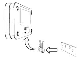
▶ Do not yet screw the antenna (1) tight in the antenna base(2) at this point. Do not use any tools for tightening.
