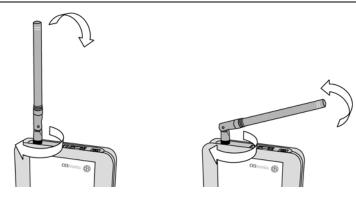
Once you have found the best position of the antenna, tighten it with your hand. Never use a tool to tighten the antenna.
